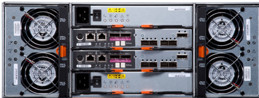
Rear View showing an enclosure with dual RAID controllers +
